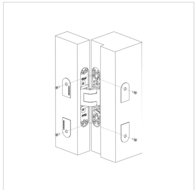
Screw the small cover plates onto the frame and door part with the enclosed, self-tapping screws.
