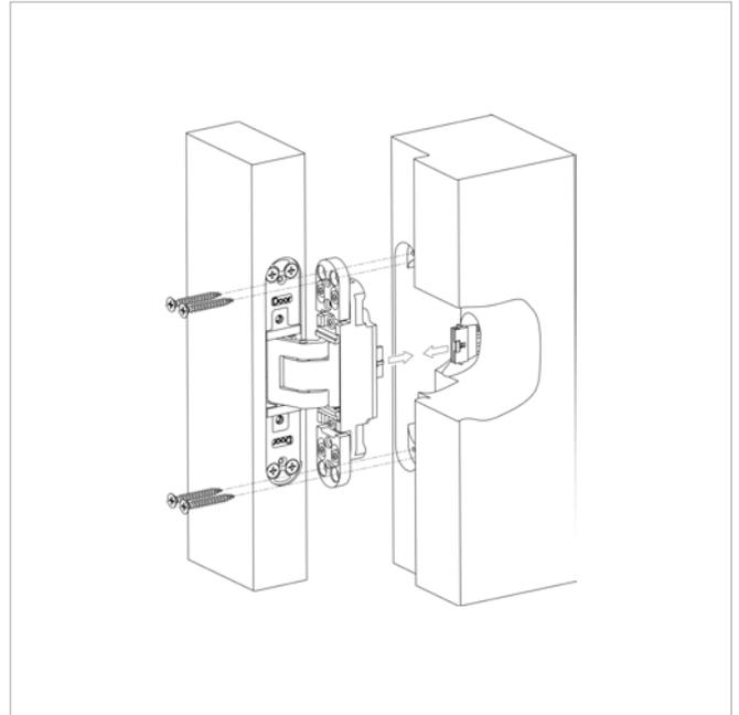
Establish the plug connection in the frame part – depending on adapter version used – and fix the frame part corresponding to frame type.
