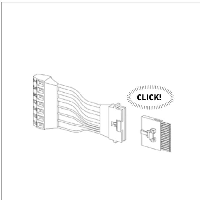
Plug connections must always click into place. Press the latch to unlock.
