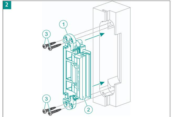
Place the hinge frame part ① in the door frame, pre-drill the door frame and fasten the hinge frame part with the four screws ③ (4.5x30 mm).
