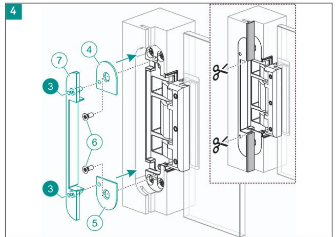
Fasten the cover plates ④ and ⑤ to the hinge with the screws ⑥. Fasten the rebate cover ⑦ with the two screws ③ flush to the frame on the cover plates. Cut the door seal to size.
