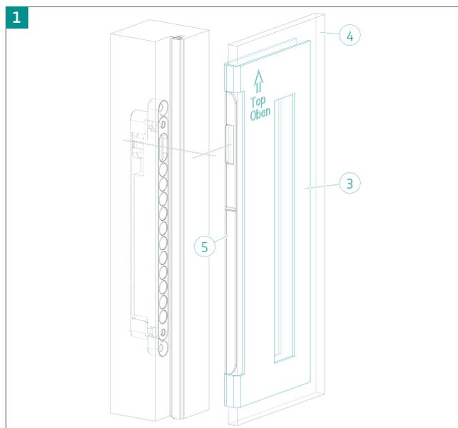
Clean the adhesive surface on the glass door ④ with the enclosed cleaning cloth.
