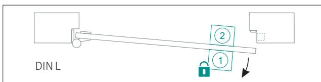
door DIN left handed, locking mechanism on the opening side
