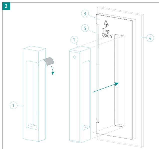
For assembly, put the KC Lock handle with locking function ① in the locked position.
