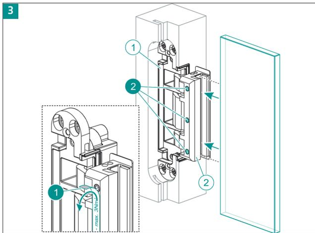
Remove the sticker ①. The clamping area must be clean and free of grease. Feed the door leaf into the hinge frame part ② as far as it will go, align in height and tighten with the three screws ② (2.5 to 3.0 Nm). Make sure there is sufficient floor clearance!
