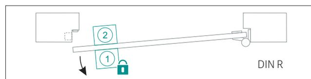
door DIN right handed, locking mechanism on the opening side
