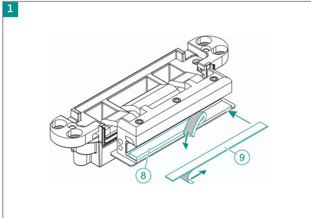
The hinge is pre-assembled for 8 mm thick door leaves. For 10 mm thick door leaves, remove the intermediate layer ⑧ without leaving any residue and glue in the intermediate layer ⑨.
