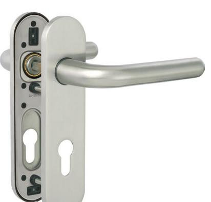
Lever set with short, invisibly fixed backplates, equipped on the female-handle face with fixed lugs. This "female" hardware is fitted on the inside of the room so as to prevent its being tampered with or dismantled. The levers are rotatably fixed on either side and are designed to cope with heavy use. The screw fixings on the outside face are concealed by an outer backplate that is securely clipped fast.
