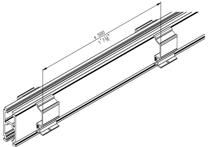
Wall mounting with spacer profile (weatherboard)
