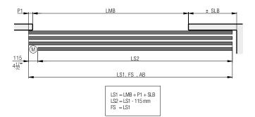
AB = System width LMB = Inside clearance SLB = Sliding shutter width P = Sliding shutter overlap LS1 = Inner running track LS2 = Outer running track FS = Guide track M = Minimum space for drive unit
