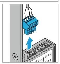
▶ Pull the green plug [1] out of the SI-BUS connection or from the analogue connection of the GENIUS.
