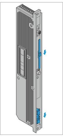
▶ Push the slider for the position inquiry [1] and the slider for the drive rod [2] into the bottom position.
