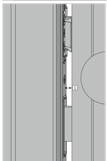
▶ In accordance with the enclosed assembly instructions of the door hinge manufacturer, adjust the airgap [1] between the faceplate and frame part.
