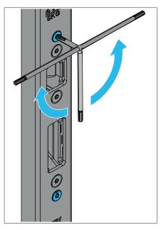
► Turn the two eccentric screws [1] to the left or right up to 90°.
