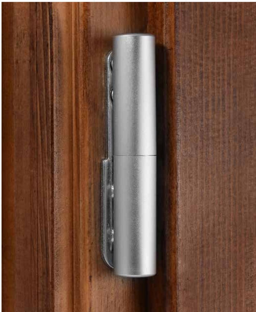
Bixacta arose from the need to have an adjustable hinge for entrance doors in PVC, wood and aluminium, which takes into account the aesthetic impact on the frame. Adjustable in 3 directions, the part fixed to the door is inserted into the euro groove axis 13 or 9 mm, air 12, the male part is interchangeable with the male Ursus or Exacta Ø16. Available in the following diameter: 16 mm.
