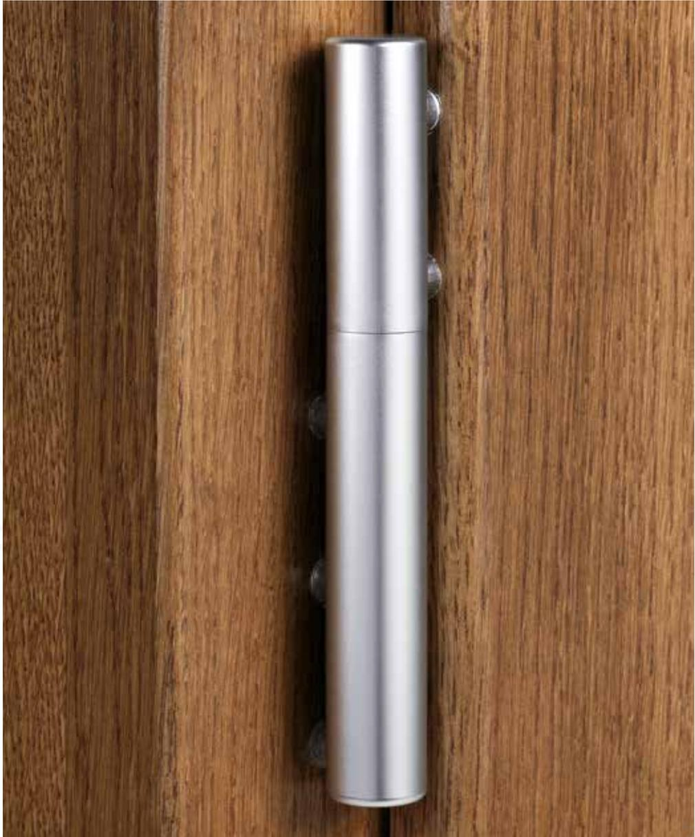
With 5 pins, this hinge guarantees high stability and carrying capacity **for particularly heavy, and very large doors**, as well as perfect alignment of the hinge. Vertical, horizontal and depth adjustments can be made. The 3 pins male part is interchangeable with several versions of Exacta hinge. Available in the following diameters: 16 and 18 mm.
