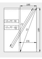
LMB = inside clearance LMH = inside height STB = sliding door width P2 = diagonal clearance LS = running track
