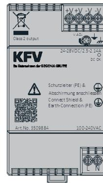
The power supply is intended for installation in the door frame (milling required), usable for GENIUS, A-opener IO modules and SIEGENIA access control systems with integrated SI-BUS adapters.
