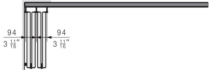
**Running gear and guide hinge**
