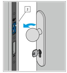
The latch [1] keeps the door closed in the released condition. It engages in the AT-piece [2] when the door is closed. The lever handle [3] is activated or the key [4] turned in the release direction up to the stop to open the door.
