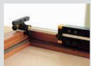
**4** • The first, easy action to drill the frame, is the correct reversible stop Positioning on the frame reference.
