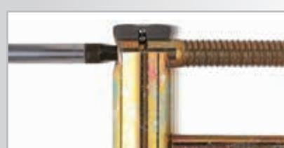
**1.** By acting on the threaded pin it is possible to quickly fit the hinge using the appropriate hexagonal bit for electrical drill screwers and then make the side precision adjustment using the special "T" wrench.
