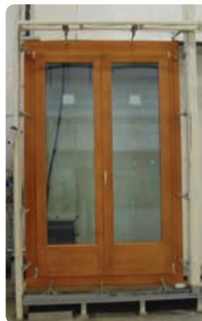
Test for resistance to water and wind
