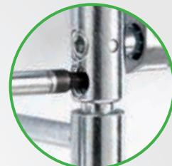
By using a "T" wrench it is possible to adjust the height of the pivot, therefore raising the female part. The weight of the door is evenly distributed over all the door-frame hinges thanks to the great sensitivity of the height adjusting device.
