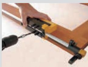
**6** • As for the door the process is the same, the correct reversible stop Positioning on the door reference, is the first operation to be done while drilling.
