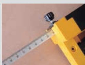
**2** • The millimetric rod allows the correct positioning of the jigs on the frames and on the doors.
