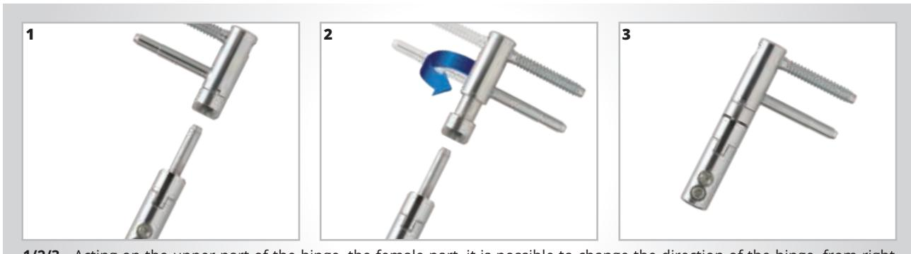
**1/2/3** - Acting on the upper part of the hinge, the female part, it is possible to change the direction of the hinge, from right to left and vice versa. It is sufficient to lift a few millimeters the movable part of the female hinge and rotate 180° to obtain a right or a left hinge.
